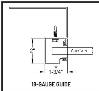
Universal mount 2" deep, 18-gauge galvanized steel guides require no pre-installation modifications for wood, steel, concrete or filled masonry block applications.
